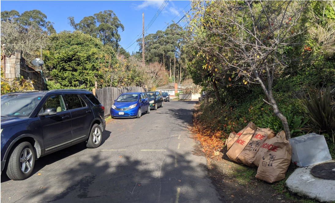
Figure 12: Lenox Road between Beverly Road and Kingston Road, looking east near the intersection of Public Path #5. The minimum width of this segment was measured to be just 11 feet, which is particularly notable given that this is a through street that could serve as an egress path for many residents of Kingston Road.
